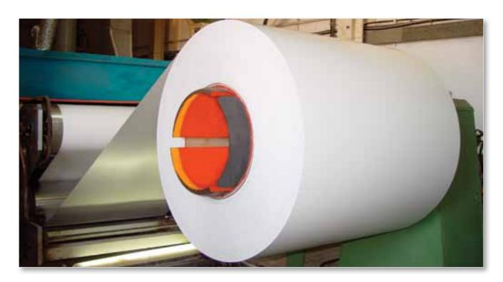
CoilCoat is a highly efficient coating plant that coats aluminum, galvanized and aluzinc coils. Three coating lines exist within the group that coat and laminate polyester, PVDF and Plastisol with embossed textures. Harwal Group uses innovative coil coating production methods and processes that generate consistent production runs. CoilCoat caters to many leading manufacturers that include roofing, cladding, composite panels, ceilings, window blinds, sporting goods and appliances.
